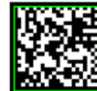
Quiet zone violation
